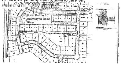
8. Add 12' asphalt pathway on south boundary of pre-plat as shown on concept plan. It is not called out on pre-plat. Extend path all the way eastward to parking lot. Place a public access easement on the pathway.
