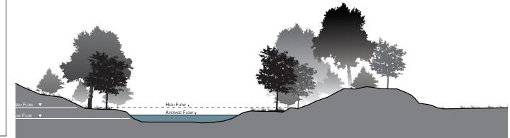
Confined Channel: Much of the river has a wide, shallow channel with that lacks structure and a thalweg (deepest portion). At low flows, the water's edge is pulled away from the banks and cover for fish and other organisms is diminished. At high flows the river is confined by levees, unable to access the floodplain.
