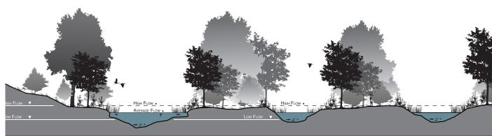
Complex River Channel: A more complex river channel with lower width to depth ratio, a well-defined thalweg, instream structure, side channels and riparian vegetation on the banks represents a target condition. At low flows, cover is provided by instream structure and vegetation; at high flows, the floodplain is accessed.
