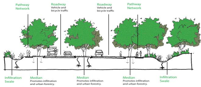
**Green boulevards** to manage stormwater. Green boulevards contain trenches and swales that promote infiltration of most urban runoff and moderate storm events. Larger storm events are moved along the swale to areas of wetlands and ponds for treatment.
