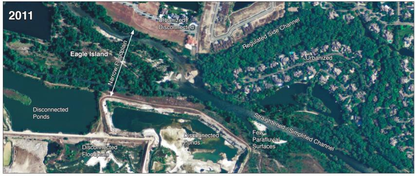
**Head of Eagle Island / River Channel 2011:** Aerial Image of the Boise River near the head of Eagle Island in 2011, more than 50 years after the completion of Lucky Peak Dam. The river channel is simplified and the floodplain disconnected and confined by urban development and flood control.
