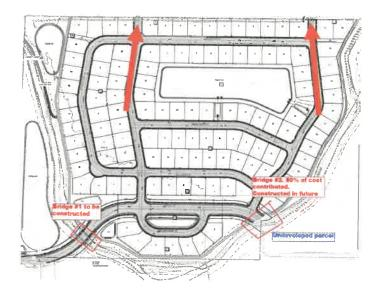
Developer's preliminary plat provides adequate stub roads to the north to allow connectivity for future development adjacent to this project. See arrows above.
