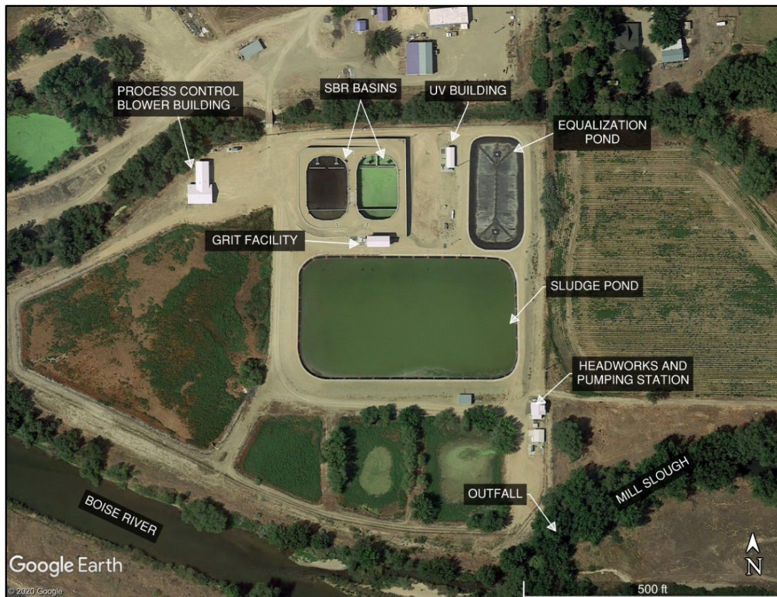
Figure 1. Middleton WWTP Existing Processes Map.
